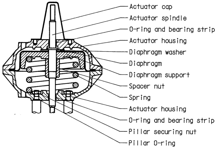
**Figure 7 Handjack Assembly - Fig. 821/861 Valve**
